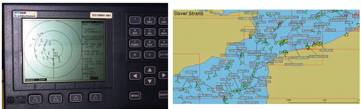
Figure 20: On-board AIS equipment and typical graphical display
